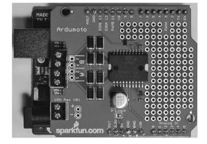
Figure 1-5 The top side of the motor shield
