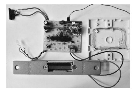
You should notice that as you connect the power, the LED should flash red, then green, and then orange twice. This is a little startup check just to show that the microcontroller chip is running.
