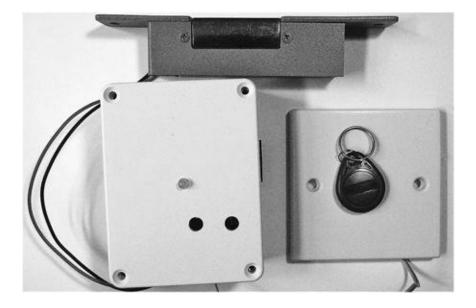
Figure 10-1 The RFID and wireless door lock
