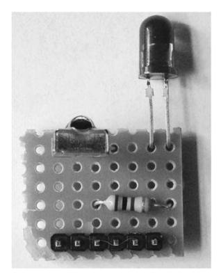
Figure 4-6 The completed stripboard
