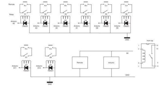
**Figure 8-3** The schematic diagram for power control
