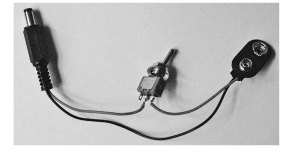
Figure 2-12 The battery lead and power socket
