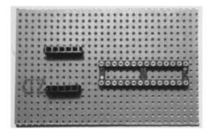
Figure 12-5 Soldering the sockets into place
