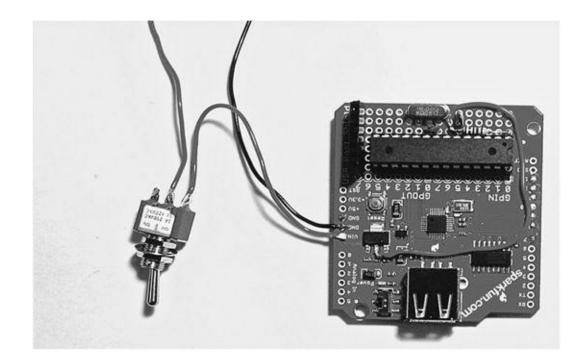
Figure 3-12 Attaching the switch and power socket
