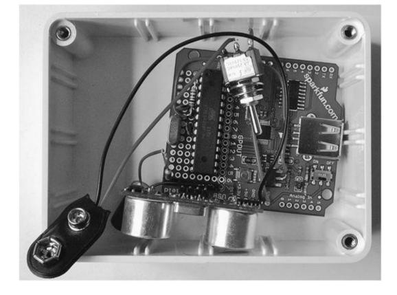
Figure 6-7 Positioning the components in the box
