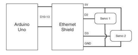
Figure 11-5 The schematic diagram for the project
