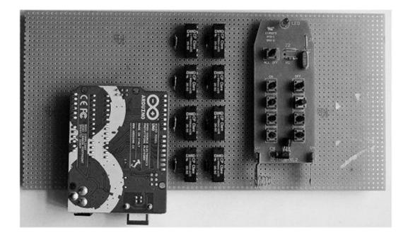
Figure 8-2 The power outlet remote control by Arduino
