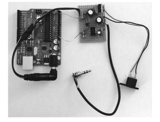
Figure 7-16 Wiring up to test the sound interface
