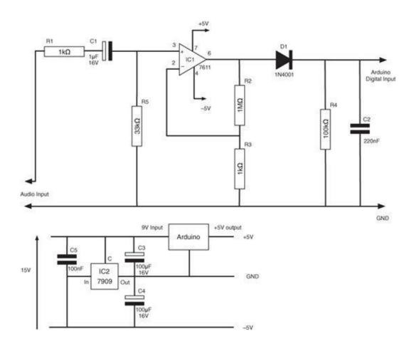
Figure 7-3 The schematic diagram for the sound link
