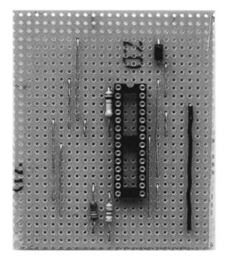
Figure 9-8 The stripboard with resistors and capacitors
