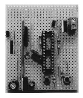
Figure 10-9 The stripboard with all the components
