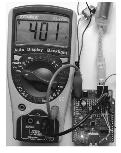
Figure 2-13 Testing the high-voltage output
