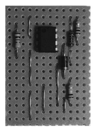
Figure 7-7 The stripboard with resistors and diode
