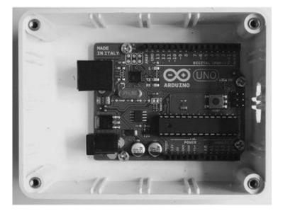
Figure 2-16 The Arduino board fixed into the box
