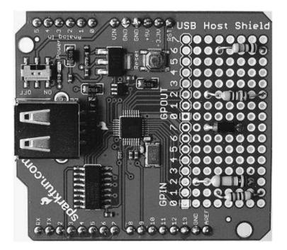
Figure 2-7 Resistors and diode on the shield
