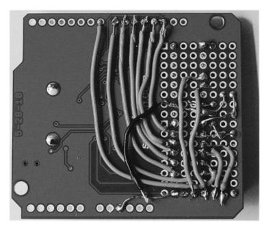
Figure 3-10 Fitting the remaining link wires
