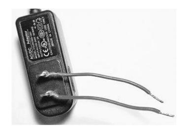
Figure 12-9 Attaching flying leads to the power adaptor
