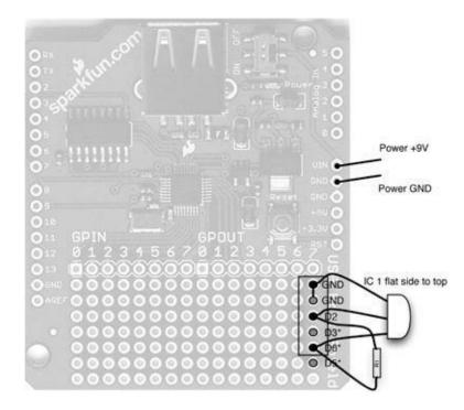
Figure 5-6 The wiring diagram
