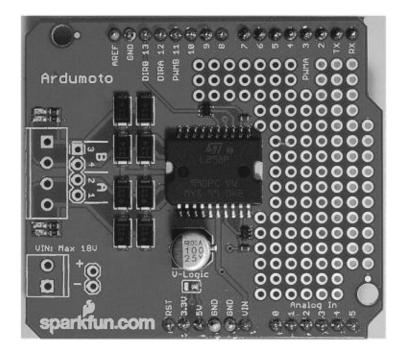
**Figure 1-6** The shield with screw terminals attached
