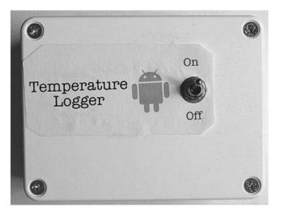
**Figure 5-1** The temperature logger Android accessory The Android control software for the project is shown in <u>Figure 5-2</u>.
