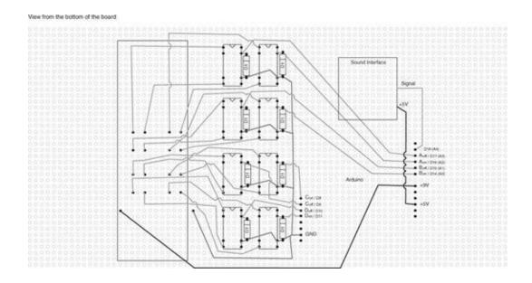
Figure 8-12 The wiring diagram with the sound interface
