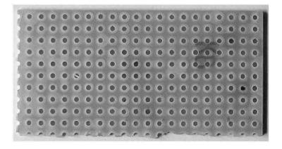
Figure 3-14 The perfboard cut to size
