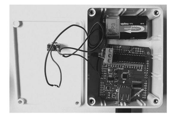
**Figure 5-8** Laying out the components in a box You will need holes for:
