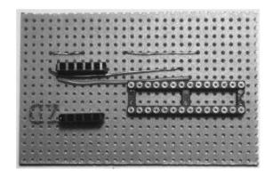
Figure 12-6 Soldering the links into place
