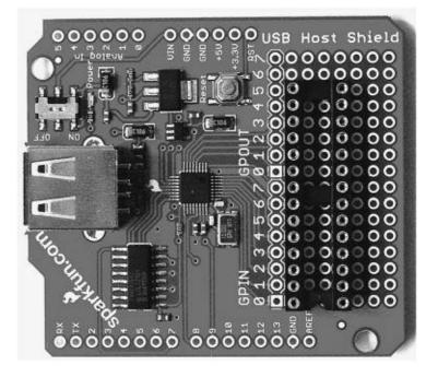
Figure 3-6 The shield with the IC socket in place
