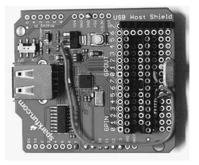
Figure 3-11 Attaching the 5V supply
