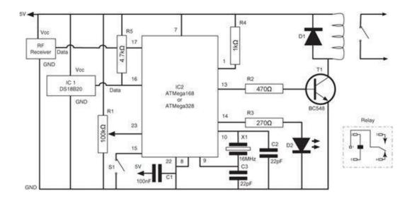
Figure 9-4 The schematic diagram for the thermostat
