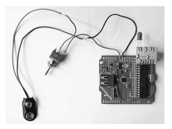
Figure 4-7 The stripboard attached to the base
