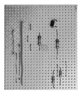
Figure 10-7 The stripboard with resistors and diode
