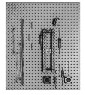
Figure 10-8 The stripboard with IC socket and switches
