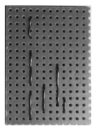
Figure 7-6 The stripboard with links
