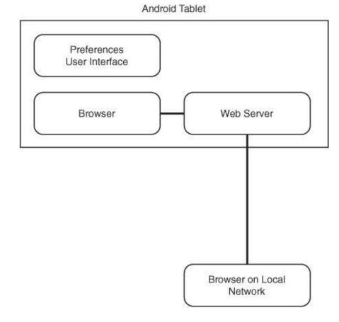
Figure 7-20 The structure of the Android app
