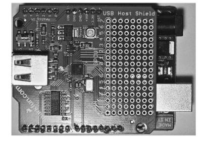
Figure 2-5 The top side of the USB shield attached to an Arduino
