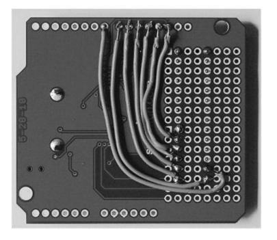
Figure 3-7 The shield with link wires attached
