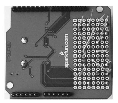
**Figure 2-9** The bottom of the board with all the components in place After that, the bottom of the board should look something like <u>Figure 2-10</u>.
