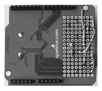
Figure 2-10 The component leads used to make connections
