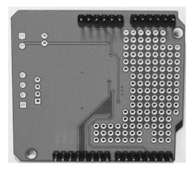
Figure 1-4 The motor shield with pin headers attached
