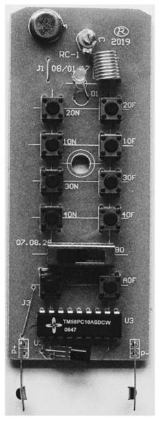
Figure 8-6 The alternative remote from the front
