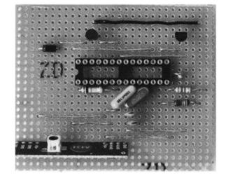
Figure 9-9 The completed stripboard
