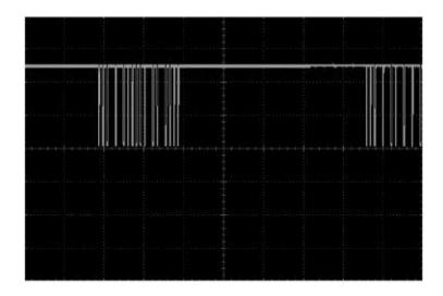
Figure 4-10 The oscilloscope trace of an IR message
