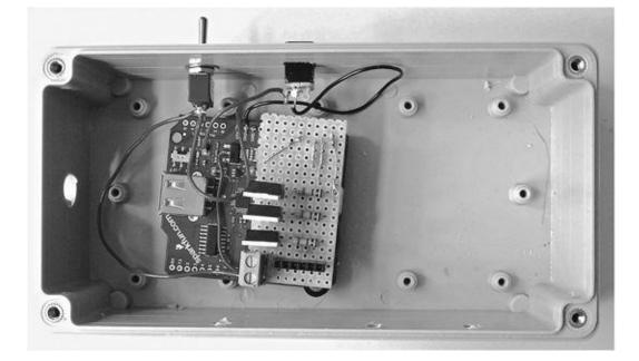
Figure 3-22 Attaching the switch and power socket
