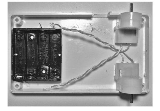
**Figure 1-8** The motors and battery box glued to the inside of the box
