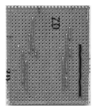
Figure 9-7 The stripboard with links
