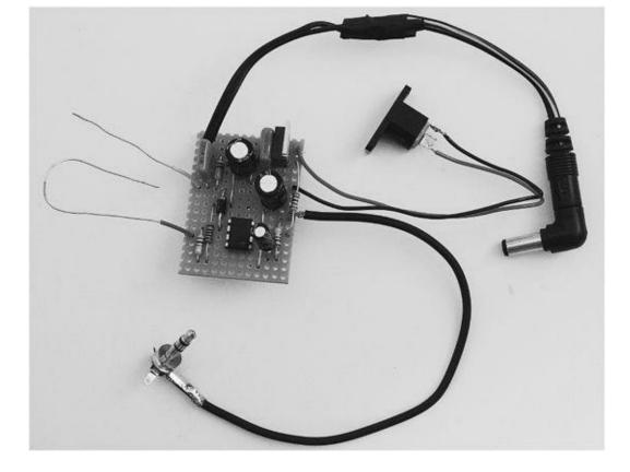
**Figure 7-10** The stripboard with trailing leads attached
