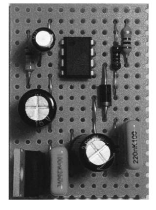
Figure 7-9 The completed stripboard
