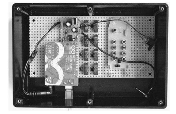
Figure 8-14 The inside of the project box with perfboard attached
