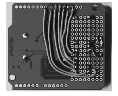
Figure 3-9 Connecting the components underneath the board
