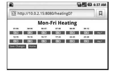
**Figure 9-2** The home automation controller—temperature control
