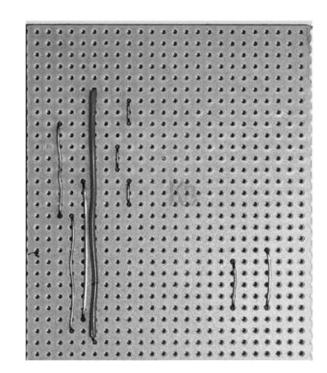
Figure 10-6 The stripboard with links in place
