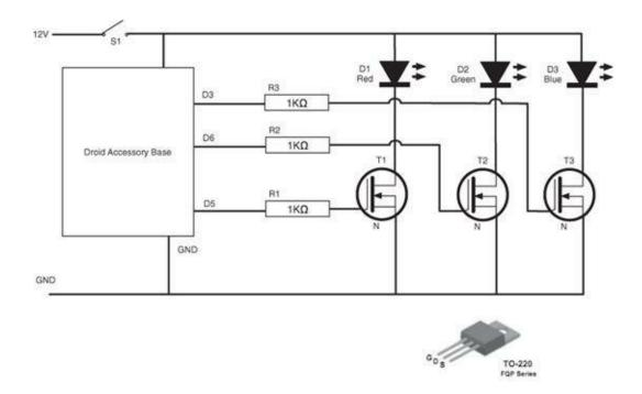
Figure 3-13 The schematic diagram for the light show itself
