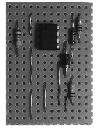
Figure 7-8 The stripboard with the IC in place
